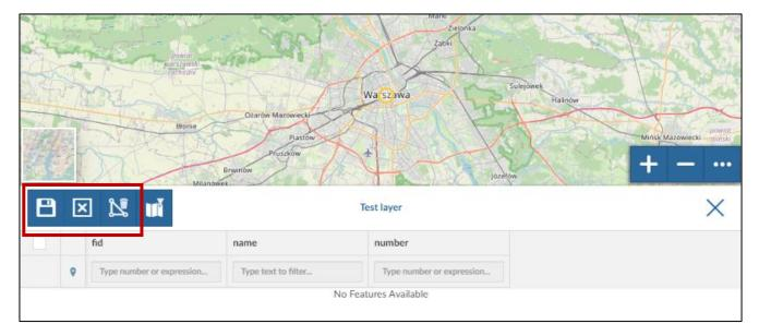
After saving the changes, the new feature is added to the attribute table below the map. Identifier (fid) is generated automatically.
